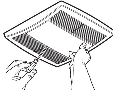
4. Remove light lens from grille by carefully inserting a small flat-blade screwdriver between grille and lens locking tab and prying lens out.
