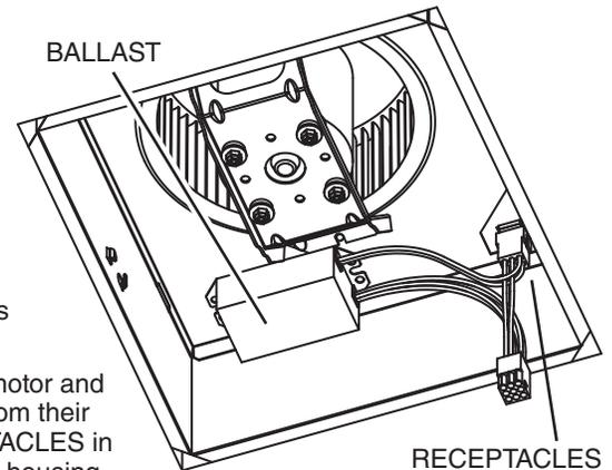
2. Remove THUMBSCREW (or hex head screw) from MOTOR PLATE FLANGE.
