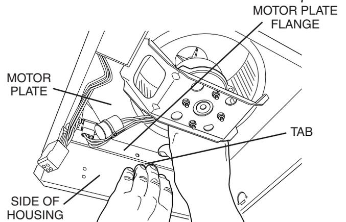
3. Find the single TAB on the MOTOR PLATE (located next to the motor's receptacle). Push up near motor plate tab while pushing out on SIDE OF HOUSING. Or insert a flat-blade screwdriver into slot in housing (next to tab) and twist screwdriver. Pivot motor plate down and remove.
