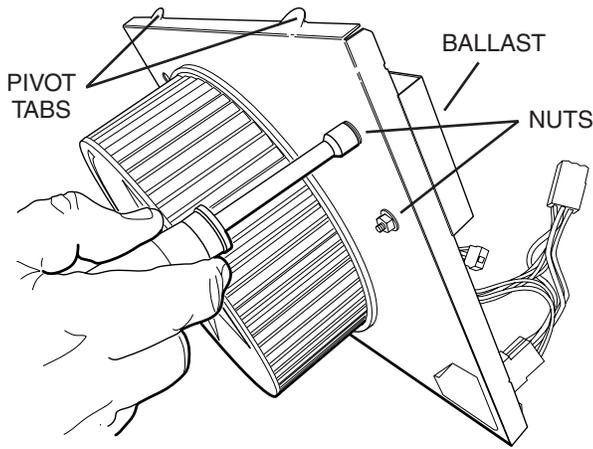
4. Remove (2) NUTS securing BALLAST using 11/32" socket or wrench. Remove ballast and dispose of appropriately, according to local laws and requirements
