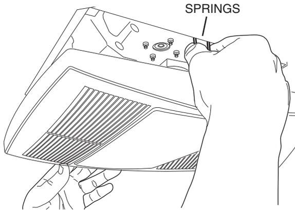
1. Pull grille assembly down from ceiling to expose two SPRINGS. Squeeze each spring together and remove from the pair of tabs on each side of housing.
