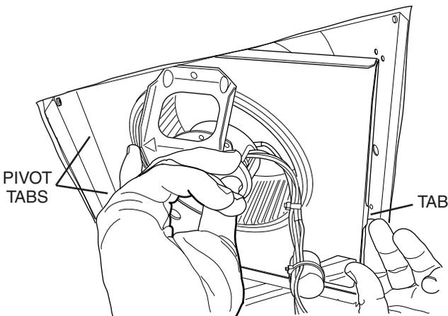
5. Reinstall blower assembly by inserting two motor plate PIVOT TABS into slots in housing and pivoting blower assembly up until the third motor plate TAB snaps into matching slot in opposite side of housing. Make sure tabs hold blower assembly securely in place.
