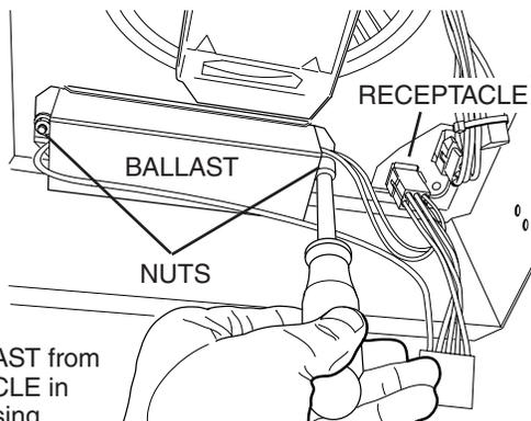
1. Unplug BALLAST from its RECEPTACLE in corner of housing.
