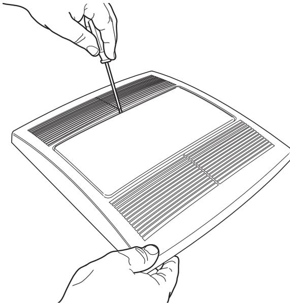
3. Remove light lens from grille assembly by inserting a small flat-blade screwdriver between grille and lens locking tab, and prying lens out.
