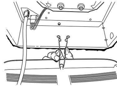
1. Plug grille assembly onto its receptacle in corner of housing.
